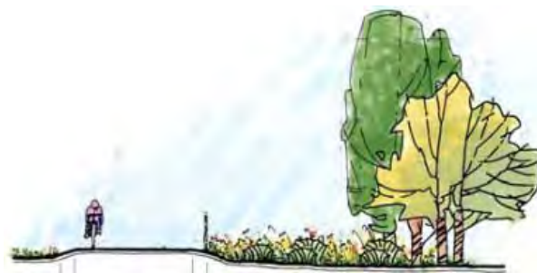
The City's Bob Jones pathway standard is a 12 foot wide asphalt pathway outside the creek setback (or an 8 foot wide pathway if within the creek setback) with 2 foot wide shoulders
