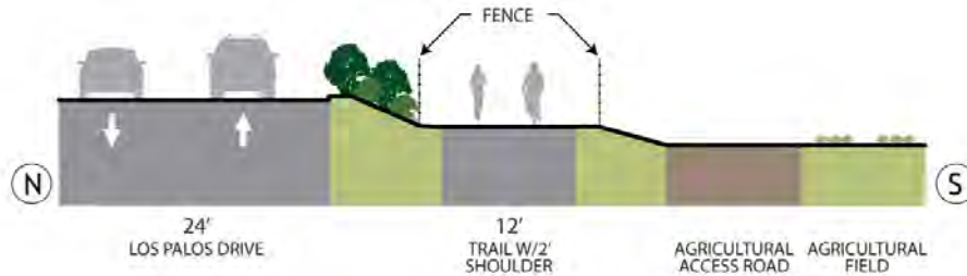
Section 3: Conceptual Cross Section Along Los Palos Drive with Pathway (facing east)
