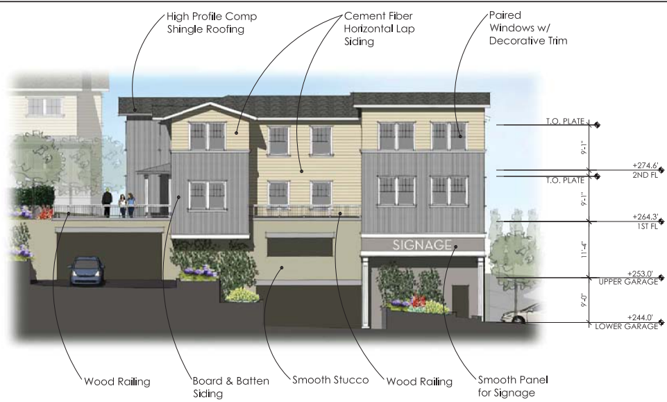
BUILDING B - EAST ELEVATION (PALOMAR AVENUE)
