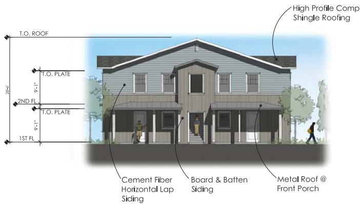
BUILDINGS C, D, E & F - FRONT ELEVATION
