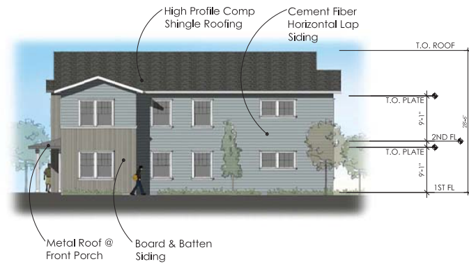
BUILDINGS C, D, E & F - SIDE ELEVATION
