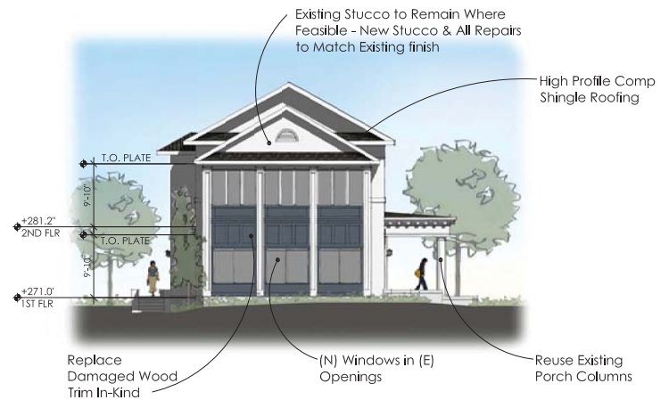
SANDFORD HOUSE - SOUTH ELEVATION (LUNETTA DRIVE)
