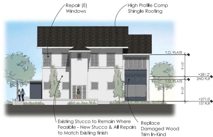
SANDFORD HOUSE - WEST ELEVATION
