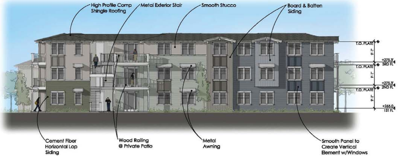
BUILDINGS B - NORTH ELEVATION
