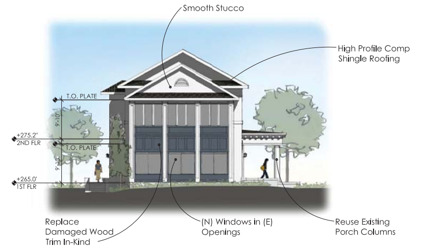
SANDFORD HOUSE - SOUTH ELEVATION (LUNETTA DRIVE)
