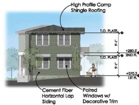
BUILDING C - WEST ELEVATION
