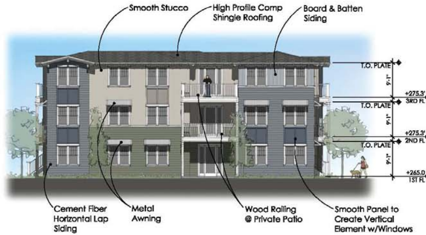
BUILDINGS B - WEST ELEVATION
