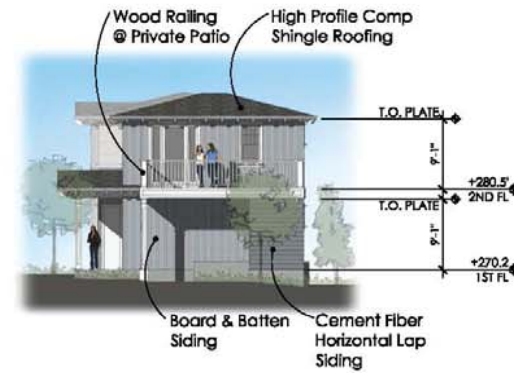
BUILDING D - EAST ELEVATION
