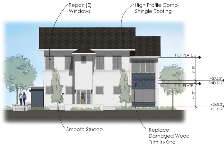
SANDFORD HOUSE - WEST ELEVATION
