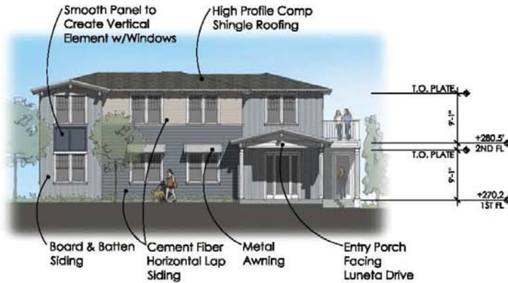
BUILDING D - SOUTH ELEVATION (LUNETA DRIVE)
