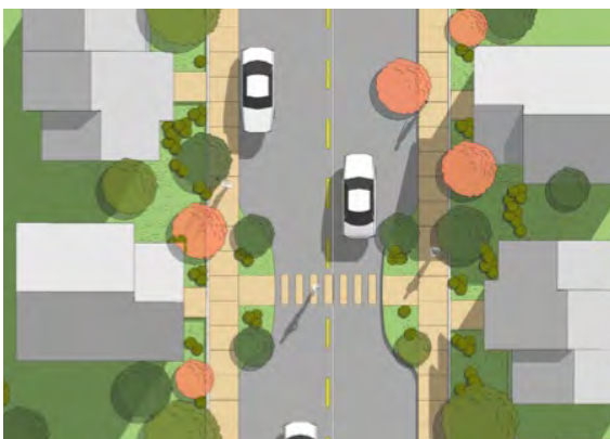
Figure 6.9 Pedestrian Crosswalks with Curb Extensions
