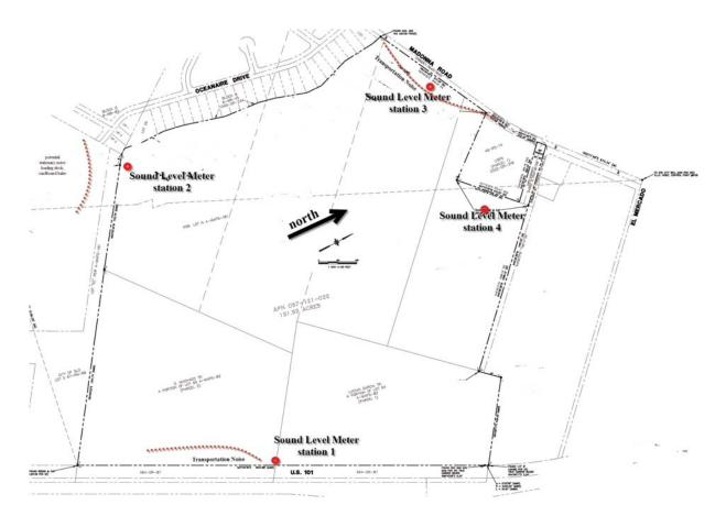
or below. If exterior sound levels exceed 60 Ldn, CAC Title 24 and the State Building Code requires the preparation of an acoustical analysis showing that the proposed design would limit the sound level to, or below the interior 45 dBA CNEL requirement.
