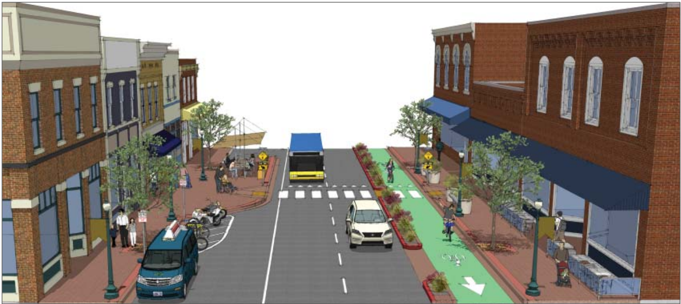
Conceptual Street Type B cross section for Marsh or Higuera Street showing a mid-block crossing with safety beacons, a passenger drop-off and loading zone, and a “smart parking” zone for bicycle and small vehicle parking.
