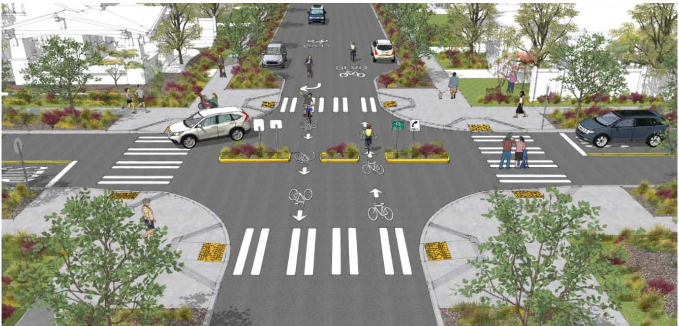
Conceptual Street Type C cross section for a typical neighborhood street intersection, including a vehicle traffic diverter.
