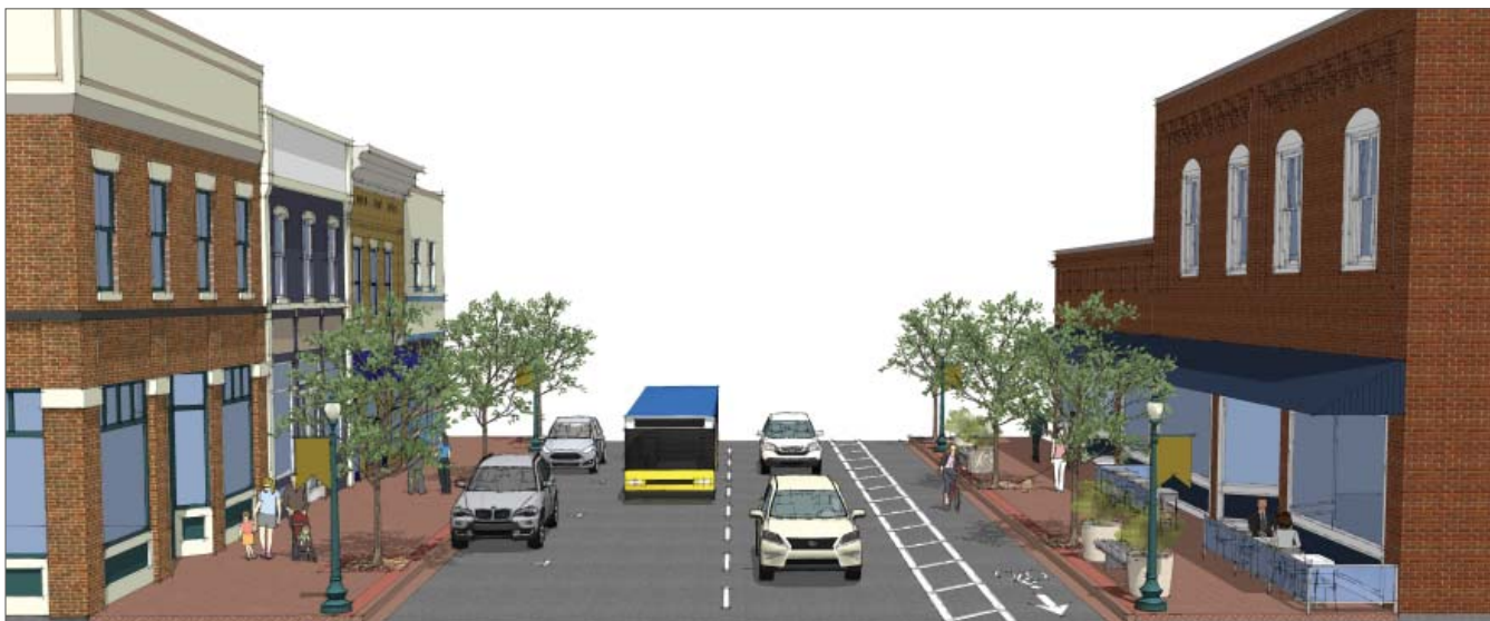
Conceptual Street Type B cross section for Marsh or Higuera Street showing two vehicle travel lanes, parking on one side of the street, a buffered bike lane, and 15' sidewalks. As shown on Figure 4.2, Bicycle Facilities Diagram, a buffered bike lane is proposed to bring bicyclists into the Central Downtown on Marsh and Higuera Streets; between Nipomo and Santa Rosa Streets it converts to a protected cycle track.
