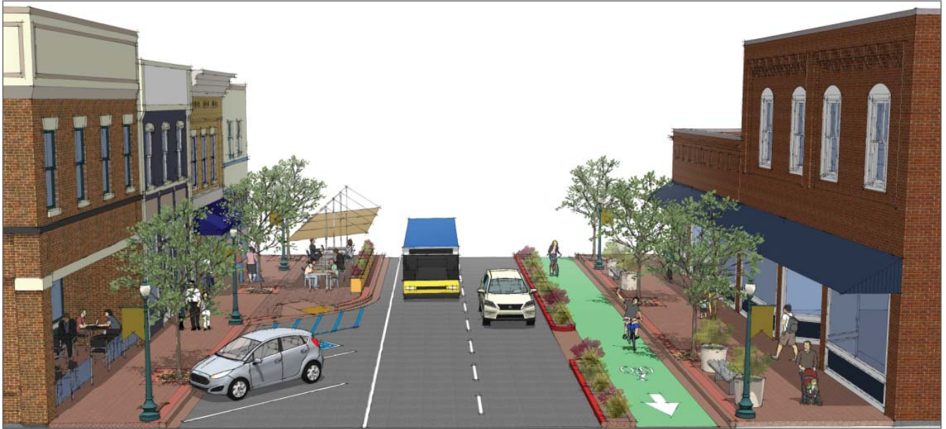
Conceptual Street Type B cross section for Marsh or Higuera Street with two vehicle travel lanes, angled parking on one side of the street, a protected cycle track, and sidewalks that widen to 24' in between parking areas, allowing for additional pedestrian experiences. As shown on Figure 4.2, Bicycle Facilities Diagram, a cycle track is proposed on Marsh and Higuera Streets in Central Downtown between Nipomo and Santa Rosa Streets.
