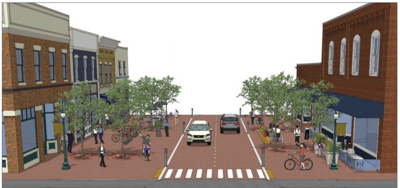
Conceptual Street Type D cross section for Monterey Street showing an ADA vision warning strip and lighted bollards to help delineate the pedestrian and vehicle zones. Pick-up and drop-off zones are allowed throughout.
