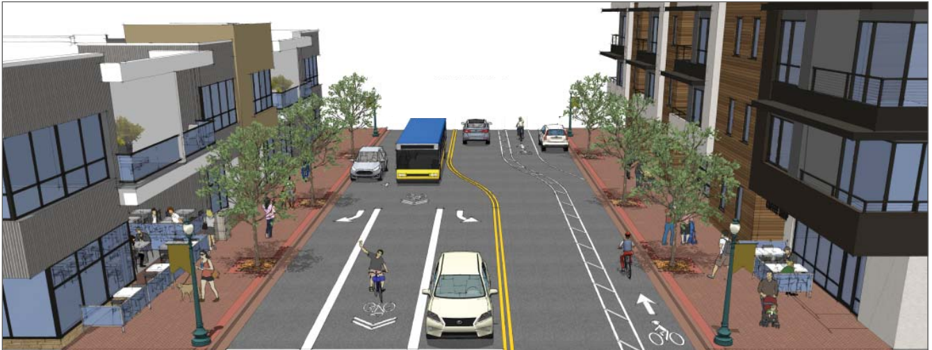
Conceptual Street Type B cross section for Monterey St in Upper Downtown, showing a buffered bike lane on the uphill and a sharrow on the downhill side of the street, parking on both sides, 12' sidewalks, and two vehicle travel lanes with turn lanes at intersections. Approximately 4' of additional sidewalk right of way is provided by adjacent businesses for enhanced outdoor dining opportunities.
