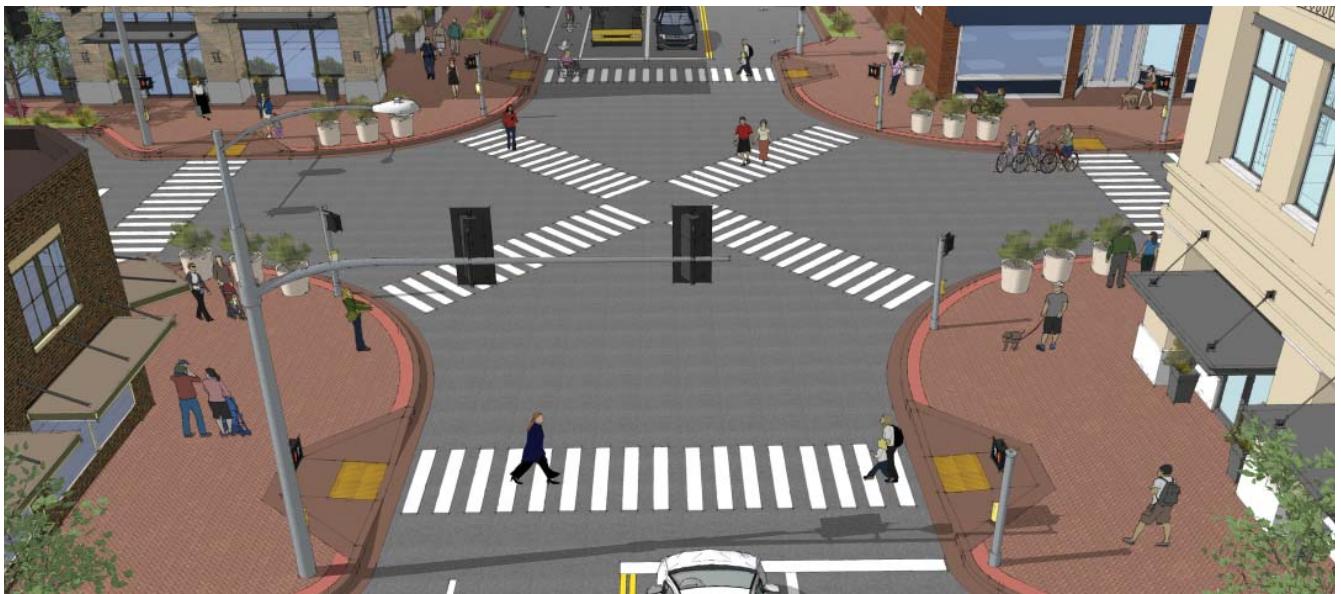
Conceptual enhanced intersection showing corner bulbouts and a pedestrian scramble.
