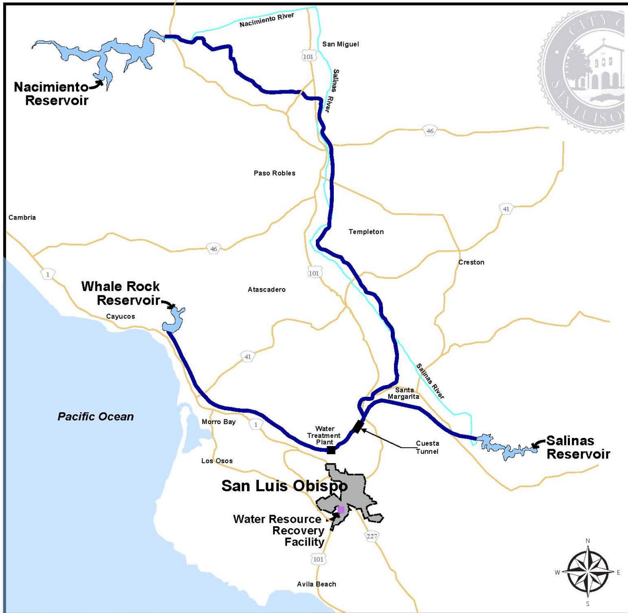
FIGURE 1: Multi-Source Water Supply Reservoir City Limits Conveyance Pipelines Source: City of San Luis Obispo Utilities Department., 2016.
