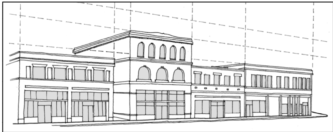
Figure 4.5 -- Horizontal lines. Reinforcing established horizontal lines is one way to provide a logical transition between adjacent buildings with different heights.
