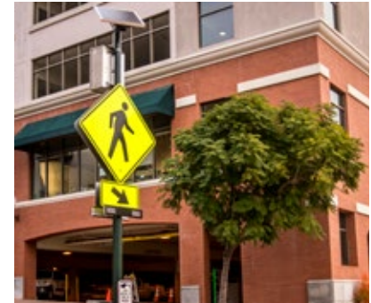
RECTANGULAR RAPID FLASHING BEACON
