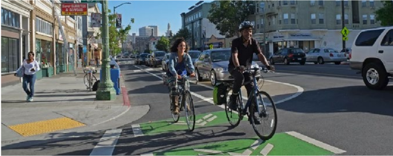
Parked cars serve as a barrier between bicyclists and the vehicle lane. Barriers could also include flexible posts, bollards, planters, or other design elements Source: Bike East Bay.
