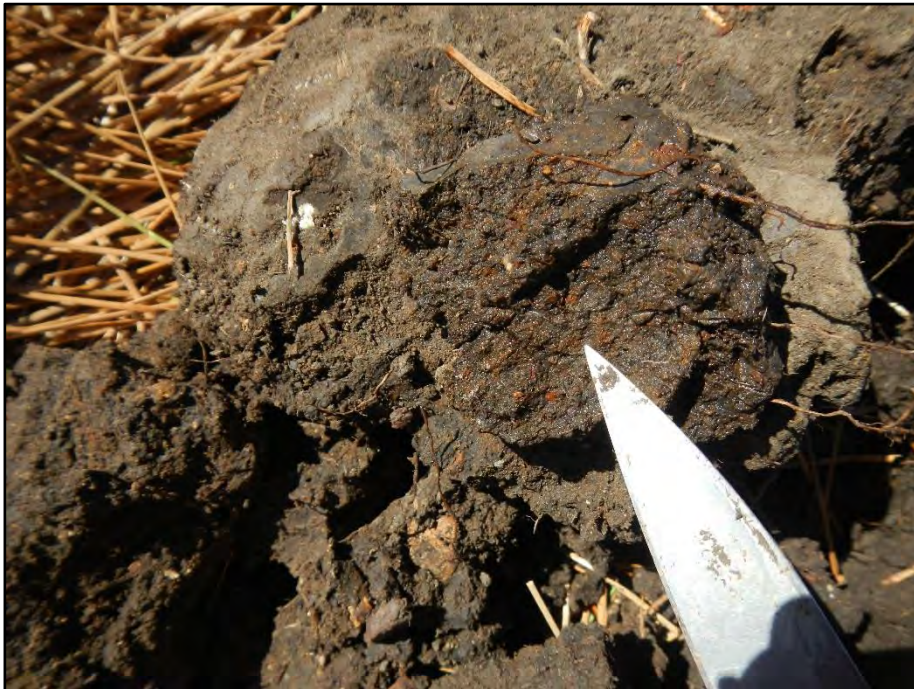
Photo 6. Soil plug from SP-05, showing redox features as oxidized pore linings along root channels (05-15-18).
