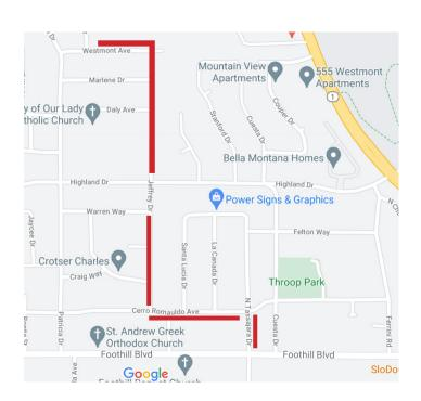
Replacement of existing gravity sewer and potable water mains at the same time will result in an overall shorter construction period as compared to replacement in multiple phases, and it will be less disruptive to traffic and residents in this area.
