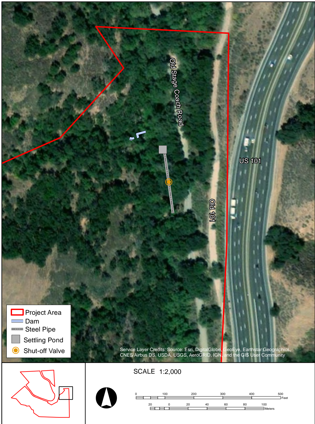
Figure 4-5 AE-4087-01H dam and associated infrastructure within the Project area.
