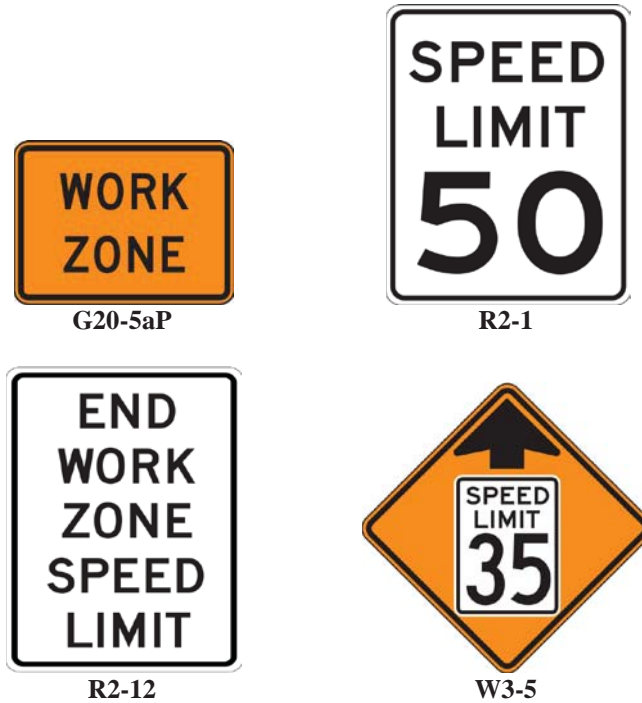
Figure 2-5: Temporary Traffic Control Regulatory Signs
