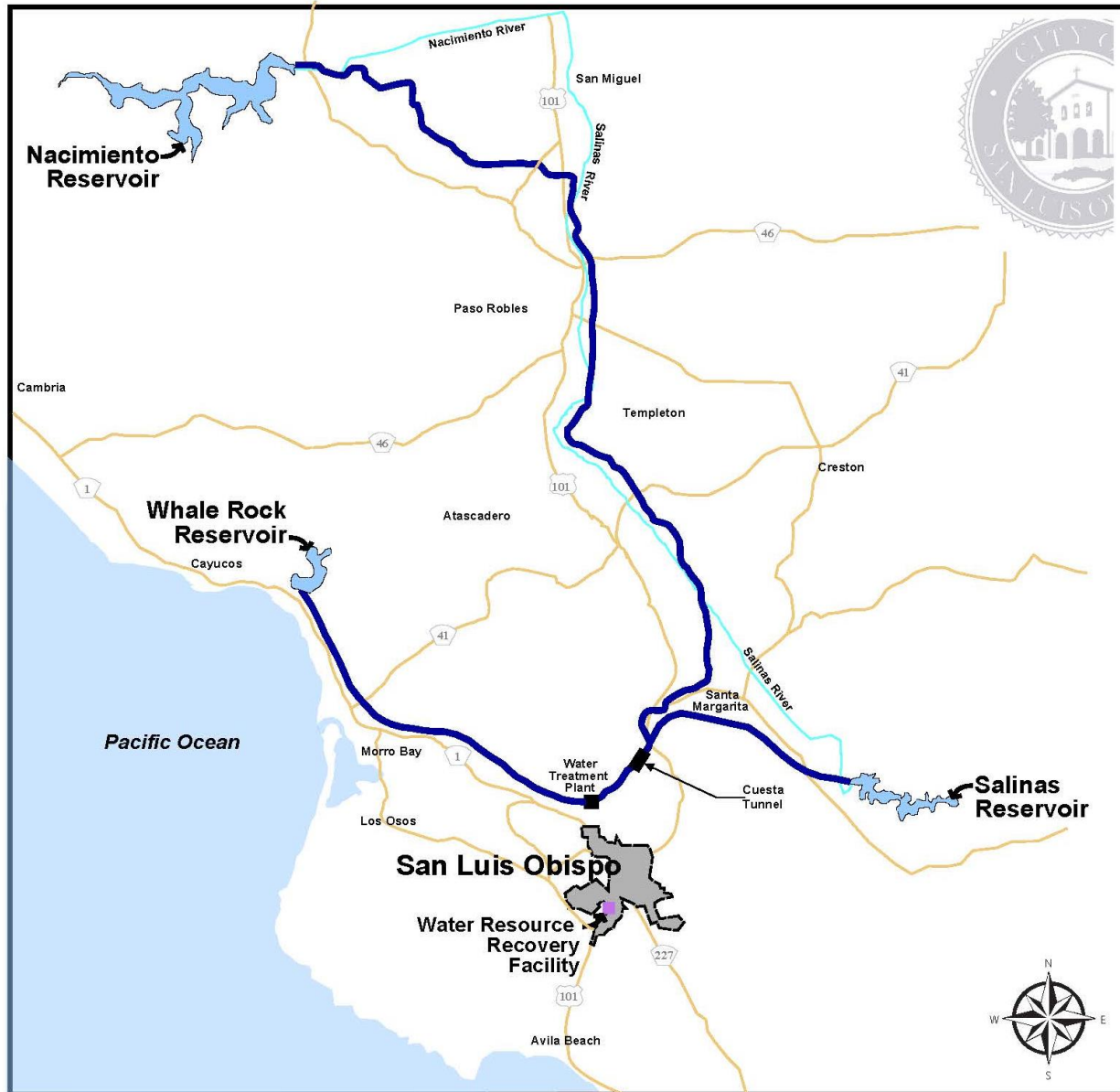
FIGURE 1: Multi-Source Water Supply Reservoir City Limits Conveyance Pipelines Source: City of San Luis Obispo Utilities Department., 2016.
